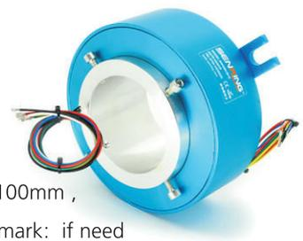
H100185 series standard precise slip ring , integrated structure design, with through hole 100mm , OD185mm , suitable for rotating application which requires a through hole <=100mm ( remark: if need a hole <100mm, can add a inner bushing)
